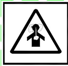
**Carbon monoxide may cause strong nausea, fainting or death. Do not use copper pipes in diesel exhaust systems. The sulphur contained in diesel exhausts causes deterioration of the system leading to exhaust gas or water leaks.**
